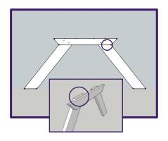
3. Next, line up the 2x6x65¾" so they are level with the ground, and the top edge extends 12½" from the legs on either side. Secure with two deck screws to hold in place.
