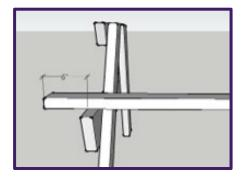
6. Next, secure the second 2x6x72" seats. Be sure to leave a ¼" gape between them. (Hint: Use a pencil to ensure a ¼" gap when attaching the seats with deck screws).
