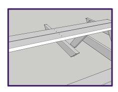
8. Then install the diagonal 2x4x32" braces flush with the center tabletop support and the seat supports (stagger slightly as shown in "Top View"). Attach with two screws at either end.
