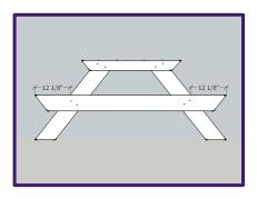
4. Attach each intersection with carriage bolts: Drill 3/6" holes and use the carriage bolts to secure the connection: keep the bolt heads against the seat and top supports (facing outward) and the washers and nuts against the legs (facing inward on a completed table). Make sure the bolts are staggered as shown.
