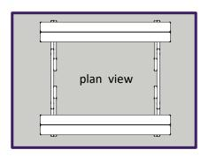
7. Attach tabletop boards and center support: (a) Lay the two (2) 2x6x72" tabletop boards on either side of the table so they overhang the A-Frames by 6". (b) Attach the 2x4x31¼" top support, parallel and centered between the A-frames, with two screws down through the tabletop boards.
