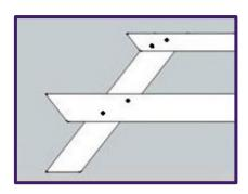
5. Attach seats: Begin by first standing up the two A-frame sides, making sure the seat supports and top supports are facing outwards and the legs are towards the inside. Then attach one (1) 2x6x72" seat on each side of the A-frames, flush with the end of the seat support. Overhang the end of the 2x6 seats 6" past the outside face of the seat support. Attach with two screw.
